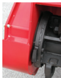
Labyrinth seals protect the rotor bearings from damage and excessive wear.
