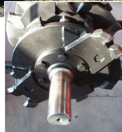
Heavy duty 80 mm diameter rotor shaft with easily interchangeable tools
